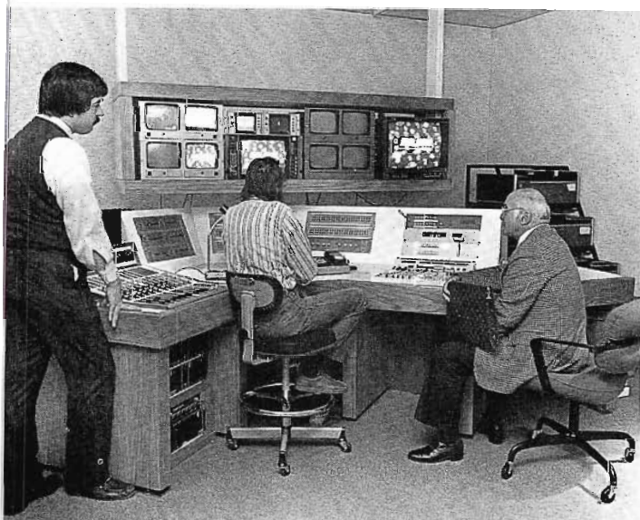
One of the three production editing rooms is equipped with a CMX editing system. This suite also includes audio mixing and video switching facilities.
