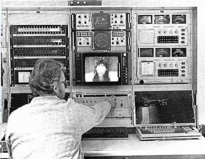
A new Transmitter Remote Control system and a computer-based control and monitoring system are a part of the Master Control Console.
